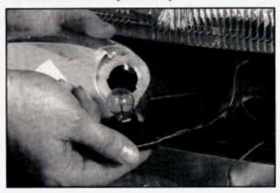
Squeeze the tab on the side of the lamp socket while turning the socket counterclockwise.
